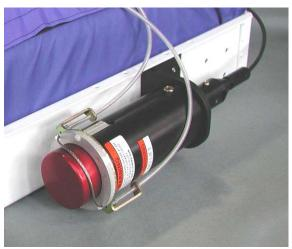
BRS-600 Launch Tube and Rocket Body (protrudes out end of tube)
